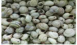
FIGURE 1. The snail shells used in biological treatment processes
