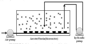
FIGURE 2. Schematic representation of the bioreactor
