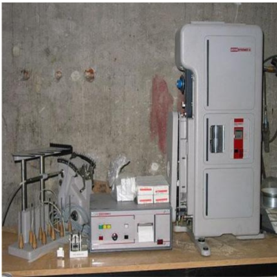
FIGURE III: A picture of Uster Dynamat II. The machine used at CSTRI for testing of silk for its tenacity and elongation.
