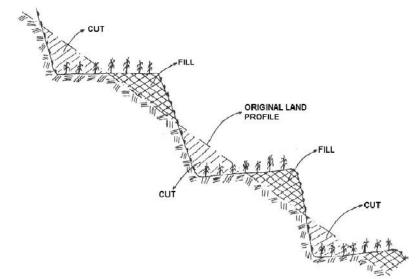
FIGURE 2. A sketch of a typical bench terrace (FAO, 2000)
