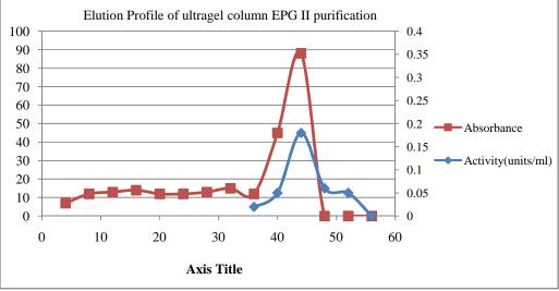
**GRAPH 7:** Elution profile of Ultragel column EPG II purification
