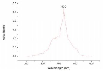
FIGURE 2. The UV spectrophotometer show the peak at 430nm indicates AgNPs formation
