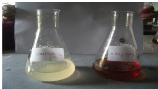
FIGURE1: Aqueous Carica papaya Fruit extract as control and bio reduction of silver nanoparticle as yellowish brown Colour.
