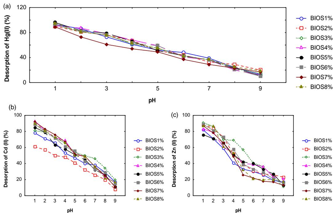
FIGURE 4. Effects of pH on desorption efficiency of (a) Hg (II), (b) Cd(II), and (c) Zn (II) from bios1 – 8.
