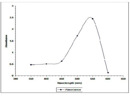
FIGURE 2: Determination of wavelength maxima ( max) of the Azo-dye, Reactive Brilliant Red X-3b at a broad wavelength scan
