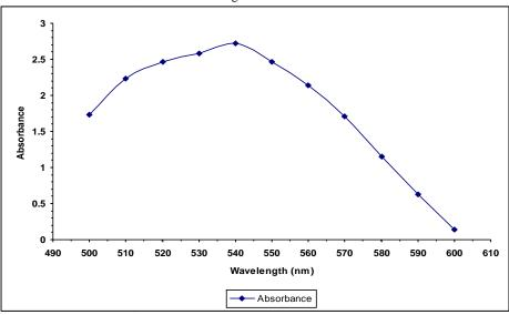
FIGURE 3: Determination of wavelength maxima ( max) of the Azo-dye, Reactive Brilliant Red X-3b at a narrow wavelength scan
