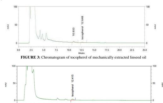
FIGURE 4: Chromatogram of tocopherol of solvent extracted linseed oil
