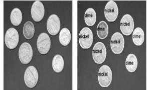
Fig 8.Object segmentation & labeling:(a) original image;(b)after segmenting & labeling individual objects.
