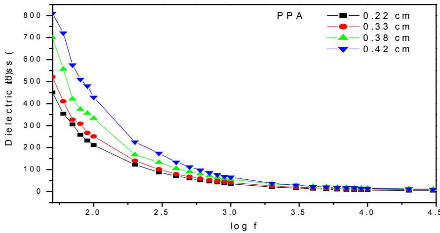
FIGURE 8- Dielectric loss of PPA as function of frequency at different thickness
