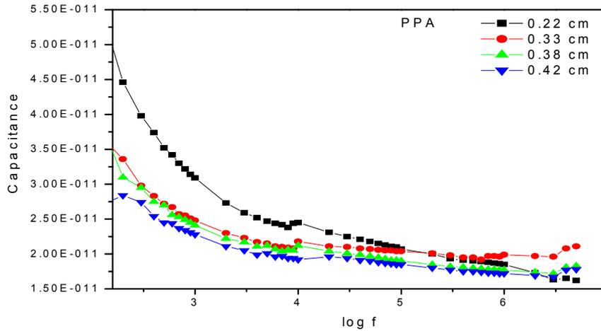
FIGURE 5 - Capacitance of PPA at different thickness as function of frequency.
