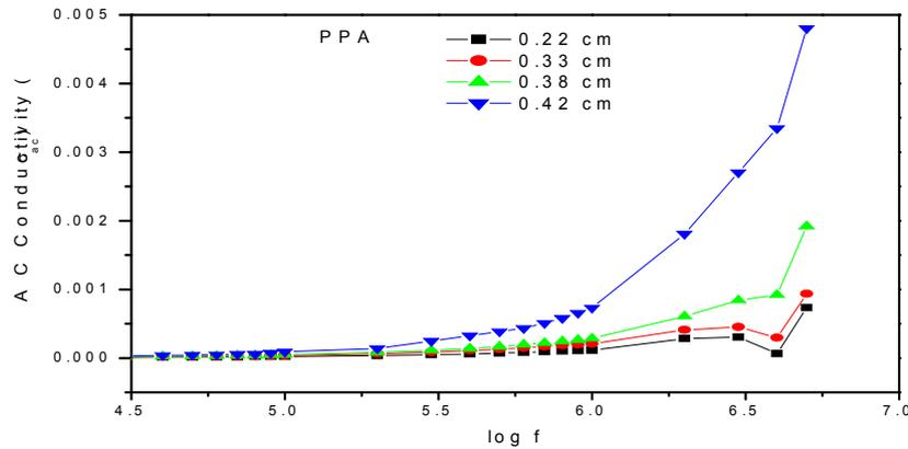
FIGURE 9 - The A C conductivity of PPA as function of frequency at different thickness.
