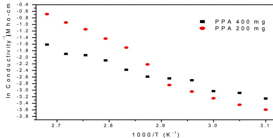
FIGURE 10 - A typical plot of  $\ln(\sigma_{dc})$  versus  $1000/T$  of PPA.
