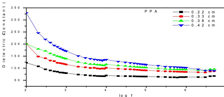
FIGURE 6- Dielectric permittivity of PPA as function of frequency at different thickness.
