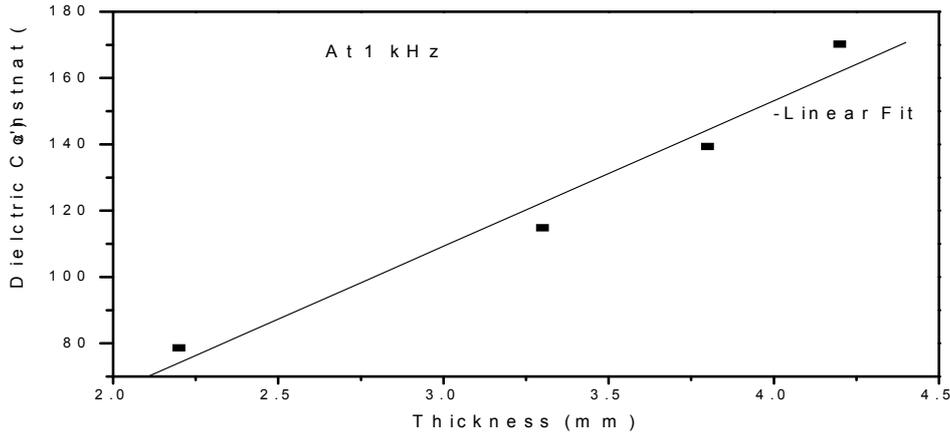
FIGURE 7- Dielectric constant of PPA at 1 KHz for different thickness.
