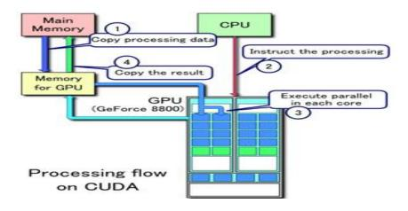
Figure 1: Processing Flow in CUDA Architecture
