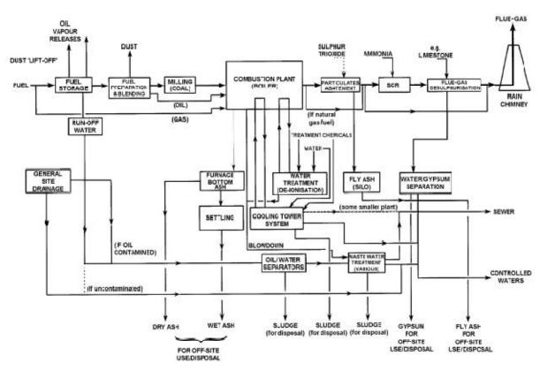
Figure 1 Flow diagram of a boiler based thermal power plant and its operations.
