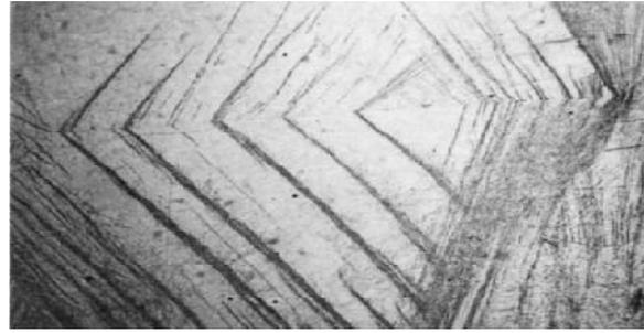
Figure 5: Slip lines in Bridgman-grown CdTe [29]
