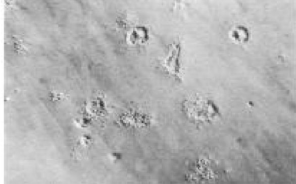
**Figure 10:** Etch pit clusters revealing dislocations generated at sites of dissolving Te precipitates (x 140) [49].
