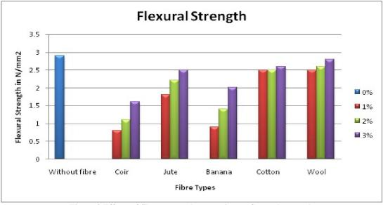
Figure 3 Effects of fibre type and proportion on flexural strength
