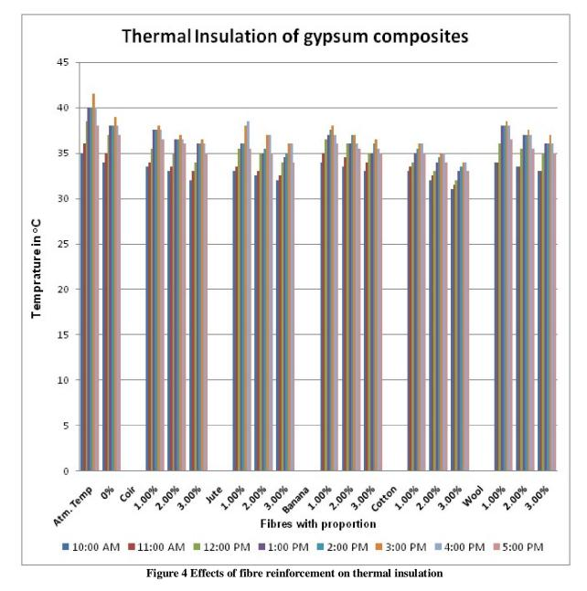
The figure 4 shows the graphical presentation of thermal insulation readings with different fiber content in the composites. On 'X' axis different fibres were plotted and
