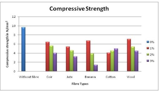
Figure 2 Effects of fibre type and proportion on compressive strength
