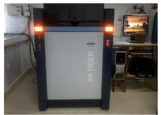
Figure 1: Picture of WDXRF setup located at Panjab University Chandigarh
