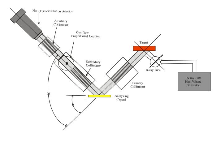
Figure 2: Schematic diagram of WDXRF setup
