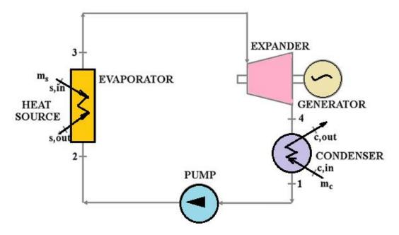
Fig. 1. Scheme of the simple ORC cycle.
