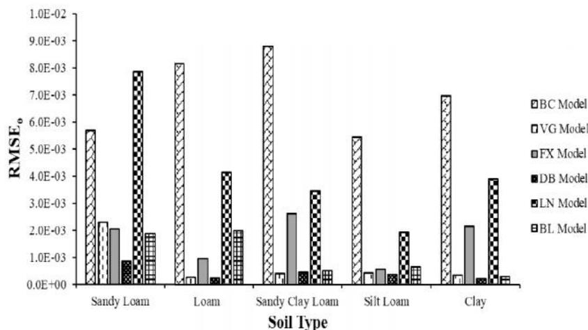
FIGURE 3. RMSE of the SWCC fitting models
