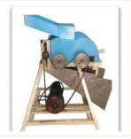
attained the required speed, jaggery was fed in to the feed hopper and operated at desired clearance. The broken jaggery was drawn into the discharge section from the
