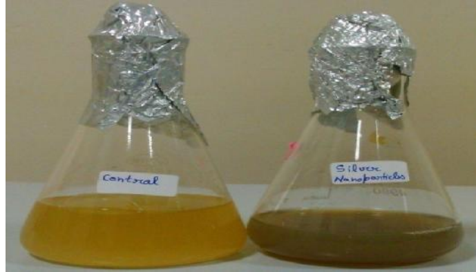
FIGURE 1: Biosynthesis of silver nanoparticles as visualized by color change from pale yellow to brown
