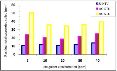
FIGURE 2: residual total suspended solid after treatment when use various doses of arabic gum for three levels of turbid water
