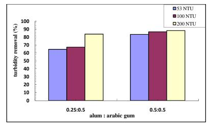
FIGURE 7: Arabic gum coagulant combine to alum with two different ratio for three levels of turbid water
