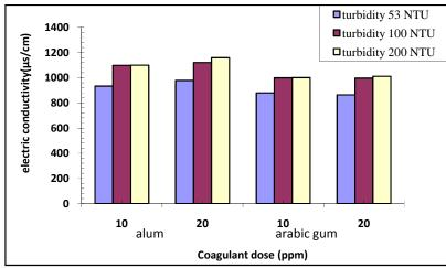
FIGURE 3: effect of alum and arabic gum coagulant at 10 and 20 ppm on electric conductivity of treated water
