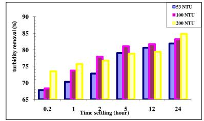
FIGURE 6: several periods of sedimentation were used in experiments for three levels of turbid water
