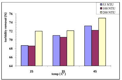
FIGURE 5: effect of three temperatures in turbidity removal for three levels of turbid water
