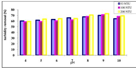
FIGURE 4: effect of pH value on turbidity removal for three levels of turbid water
