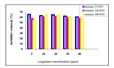
FIGURE 1: effect of various doses of arabic gum on water turbidity removal for three levels of turbid water
