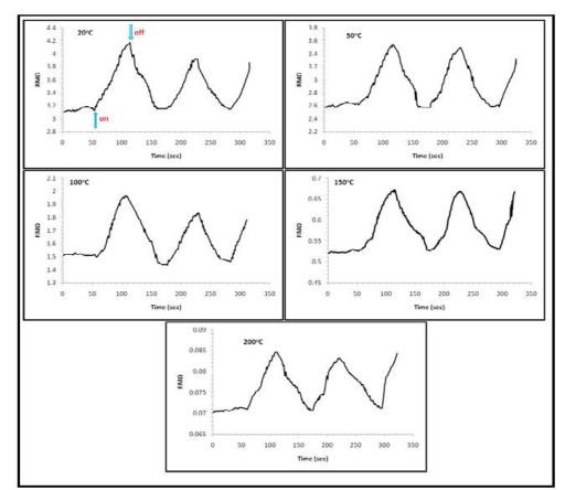
FIGURE 8: The Variation of resistance with time to PPy and 0.01% fSWCNT) at different operation temperature
