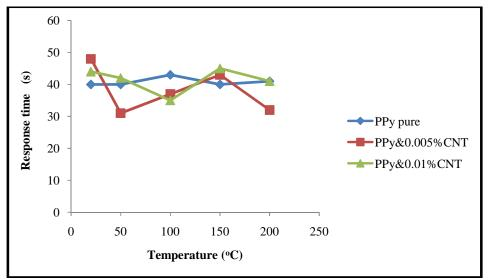
FIGURE 10: The variation of Response time with operating temperature of PPy and PPy/fSWCNT films
