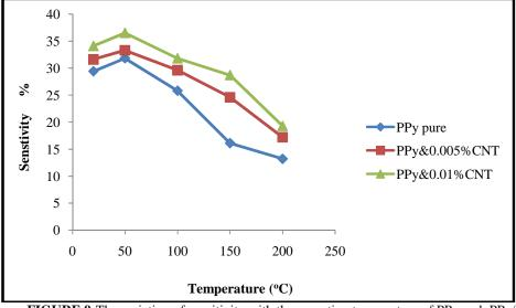
FIGURE 9: The variation of sensitivity with the operating temperature of PPy and PPy/fSWCNT films
