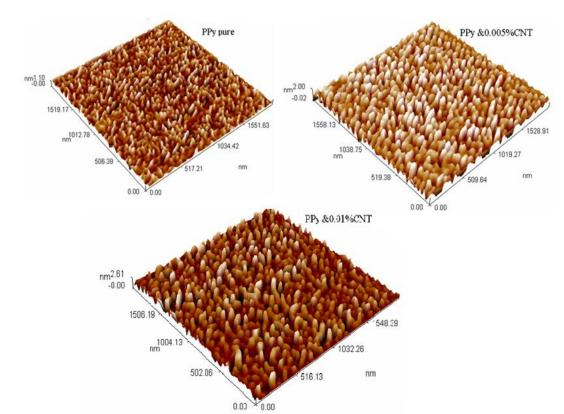
FIGURE 3. 3-D AFM image of nanostructured PPy and (PPy/fSWCNT) films
