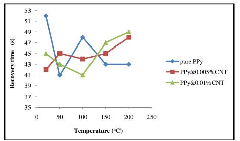
FIGURE 11: The variation of Recovery time with operating temperature of PPy and PPy/fSWCNT films
