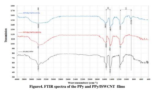
In the spectra of Pure PPy, a broad absorption band obtained a stretching N-H band at 3416.21 cm<sup>-1</sup>. The bands at (1558.52 and 1452.82) cm<sup>-1</sup> is related to the C=Cstretching mode, and the bands at 1176 cm<sup>-1</sup> is associated to the C-H bending modes while the band for C-H out-of-plane deformation vibration was observed at
