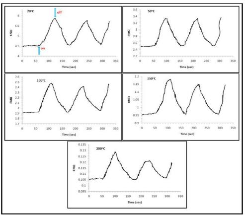
FIGURE 7: The Variation of resistance with time to PPy and 0.005% fSWCNT at different operation temperature
