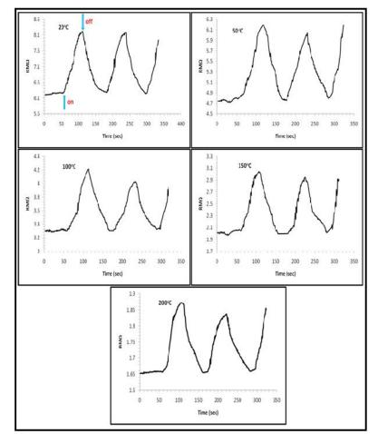
FIGURE 6: The Variation of resistance with time to pure PPy at different operation temperature
