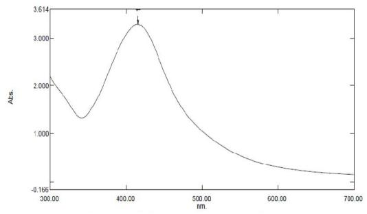
FIGURE 3: UV-Vis absorption spectra of silver nanoparticles synthesized by Drymoglossum piloselloides
