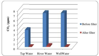
FIGURE 11: Mean Carbonate Ions Value (ppm) of Water Samples before/after Treatment
