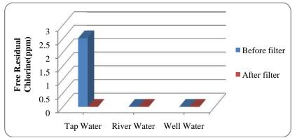
FIGURE 5: Mean Free Residual Chlorine Value (ppm) of Water Samples before/after Treatment
