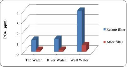
FIGURE 9: Mean Phosphate Ions Value (ppm) of Water Samples before/after Treatment
