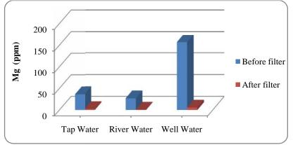
FIGURE 7: Mean Magnesium Ions Value (ppm) of Water Samples before/after Treatment
