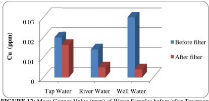
FIGURE 12: Mean Copper Value (ppm) of Water Samples before/after Treatment
