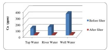
FIGURE 6: Mean Calcium Ions Value (ppm) of Water Samples before/after Treatment
