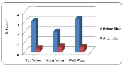
FIGURE 8: Mean Potassium Ions Value (ppm) of Water Samples before/after Treatment
