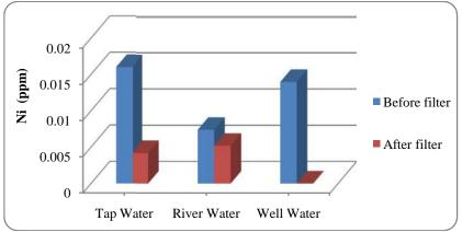
FIGURE 13: Mean Nickel Value (ppm) of Water Samples before/after Treatment
