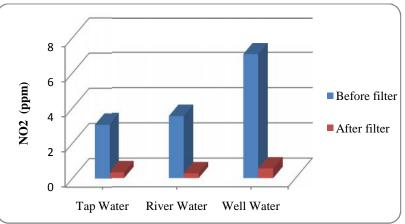
FIGURE 10: Mean Nitrite Ions Value (ppm) of Water Samples before/after Treatment
