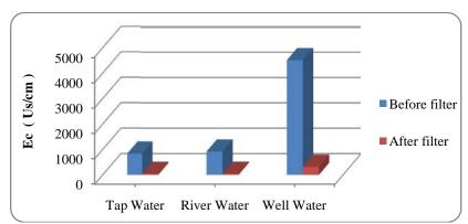
FIGURE 3: Mean Electrical Conductivity Value (µs/cm) of Water Samples before/after Treatment
