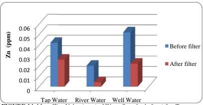
FIGURE 14: Mean Zinc Value (ppm) of Water Samples before/after Treatment
