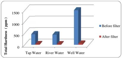
FIGURE 4: Mean Total Hardness Value (ppm) of Water Samples before/after Treatment
