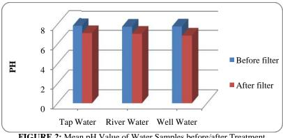
FIGURE 2: Mean pH Value of Water Samples before/after Treatment
