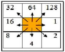
FIGURE 11: flow direction
