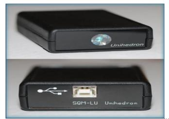
FIGURE 5: Sky Quality Meter; model LU (front and back of unit)<sup>[14]</sup>
