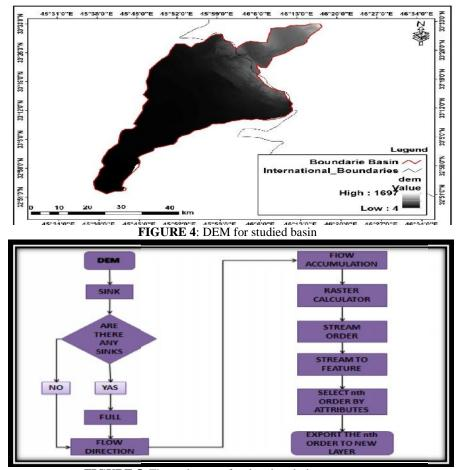
FIGURE 5: The main steps for drawing drainage pattern
