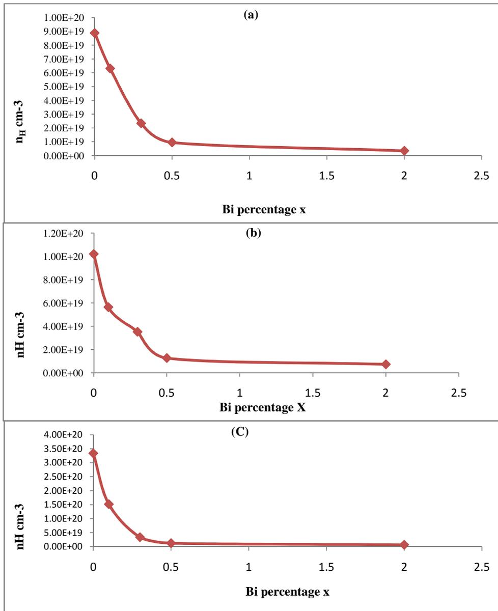
FIGURE 4: the relation between carrier concentration  $n_H$  as a function of (Bi) percentage(X) of  $(Bi_2Sb_{2-x}Te_3)$  thin films for the : a-(100nm),b-(300nm), and c- (500nm).
