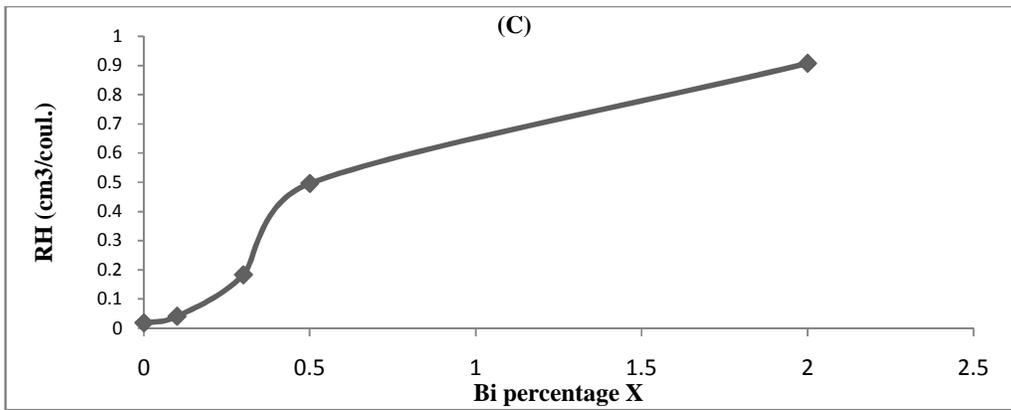
FIGURE 3: The relation between Hall coefficient  $R_H$  as a function of (Bi) percentage(X) of  $(Bi_2Sb_{2-x}Te_3)$  thin films for the : a-(100nm),b-(300nm), and c- (500nm).
