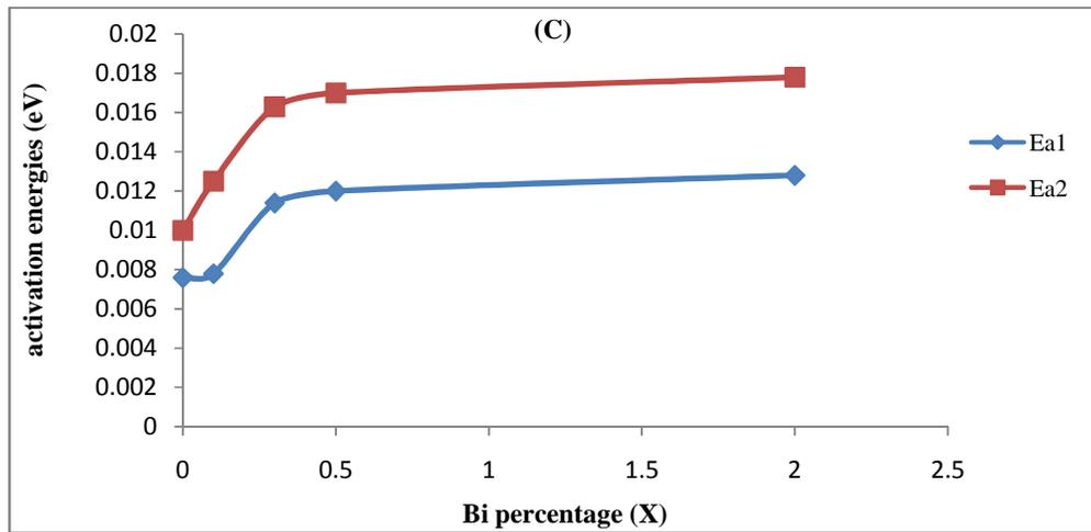
FIGURE 2: The variation of activation energies with Bi percentage for (Bi<sub>x</sub>Sb<sub>2-x</sub>Te<sub>3</sub>) thin films for: a-(100nm) ,b-(300nm), and c-(500nm)
