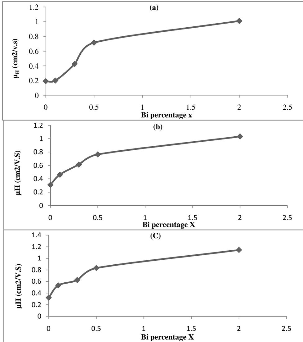
FIGURE 5: The relation between hall mobility ( $\mu_H$ ) as a function of (Bi) percentage(X) of ( $\text{Bi}_x\text{Sb}_{2-x}\text{Te}_3$ ) thin films for the : a-(100nm),b-(300nm), and c- (500nm).
