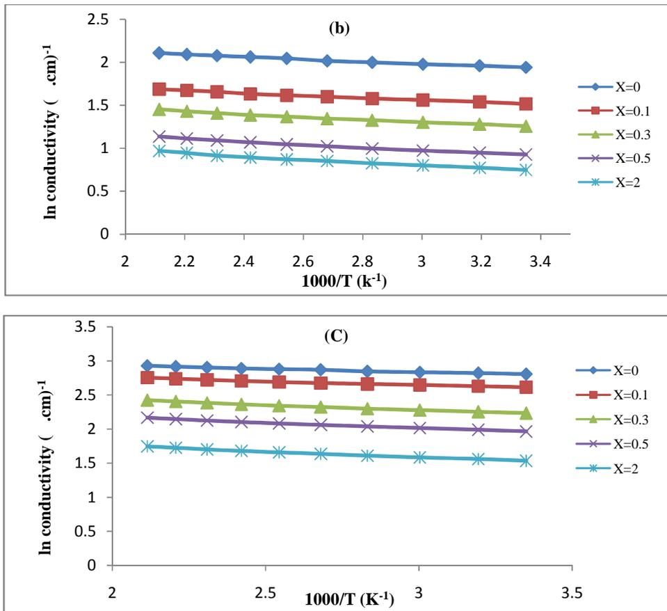
FIGURE 1 : The nature logarithm of electrical conductivity as a function of 1000/T for  $(\text{Bi}_x\text{Sb}_{2-x}\text{Te}_3)$  thin films for : a- (100nm) ,b-(300nm), and c-(500nm)
